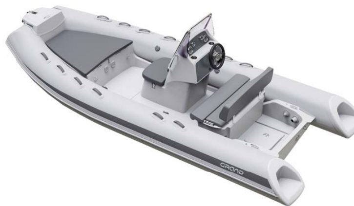
S520LF - DELUXE version with optional bow step plate, bow cushion and fiberglass step ends on tube
