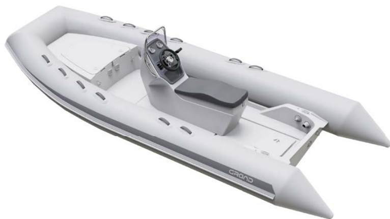
S520S - SPORT version with CS-03 console with windshield and handrail
